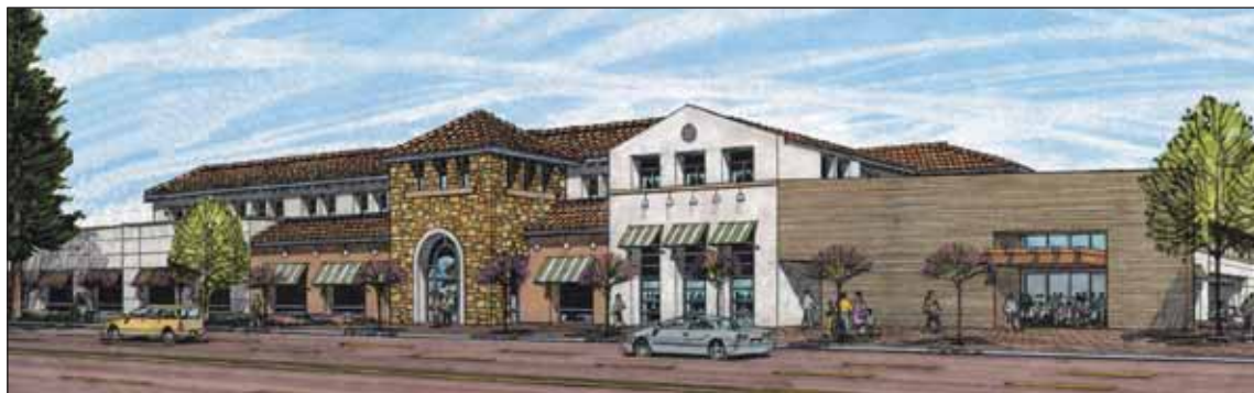
An architect's rendering of the 110,000 square-foot office/retail project proposed for 1300 El Camino Real. The structure would be set back from the curb by 22 feet for most of its length, and would reach a height of 40 feet.
