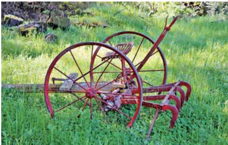
This ride-along cultivator includes a lever-handle to raise and lower the blades as they dig into the soil of a plowed field.
