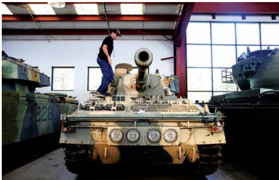
This British fighting vehicle being inspected by Ken Howe may look like a tank, but this FV433 Abbot 105 mm self-propelled gun has no rotating turret.
