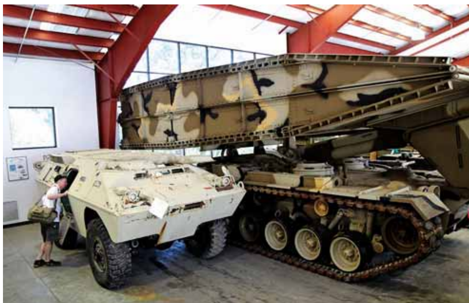
This light tan Dragoon (left), an American armored personnel carrier, had a crew of three and could carry six infantry soldiers. Next to it is a mobile bridge, also American.
