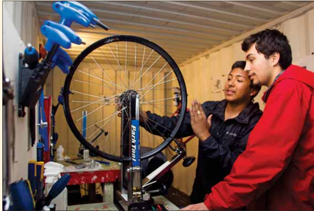
Left: Juan Rivera, left, shows Brian Palominos how to "true" a wheel during a bicycle-repair class. Below: Teacher Dan Hensley explains to Juan Rivera what happens when you adjust the tension on individual spokes.
