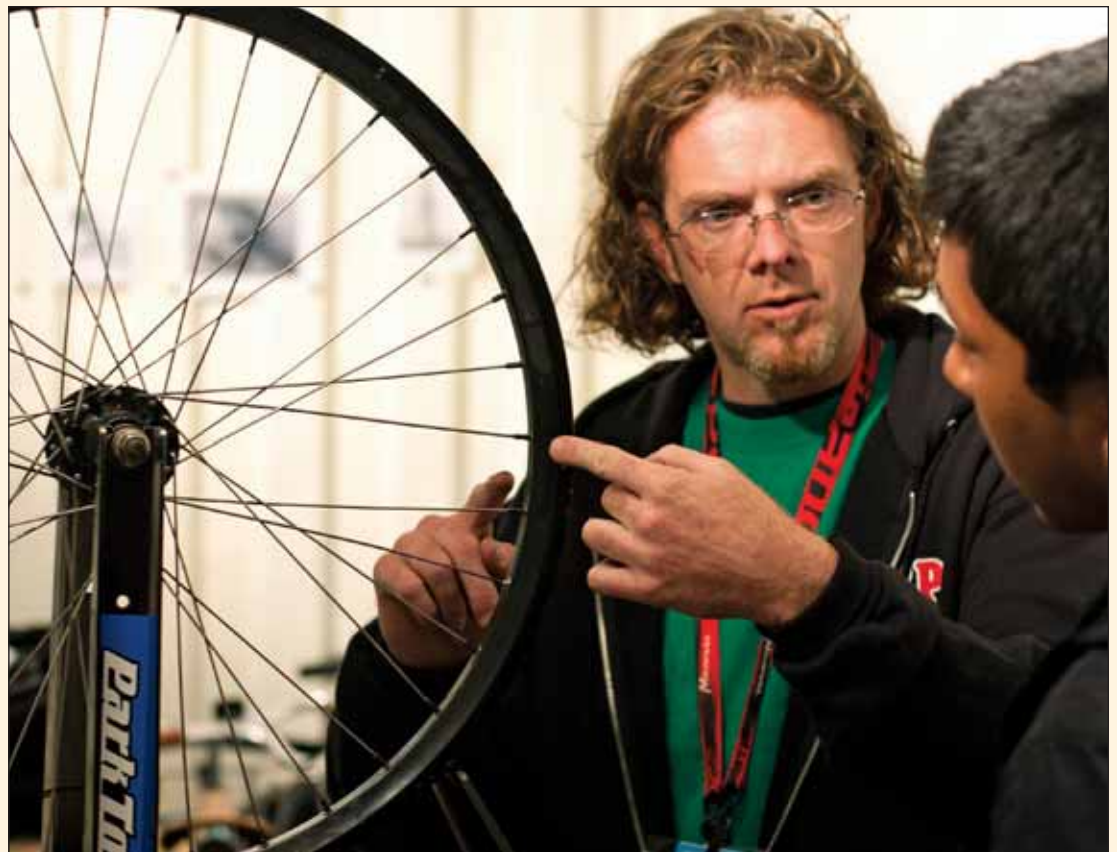
Left: Juan Rivera, left, shows Brian Palominos how to "true" a wheel during a bicycle-repair class. Below: Teacher Dan Hensley explains to Juan Rivera what happens when you adjust the tension on individual spokes.
