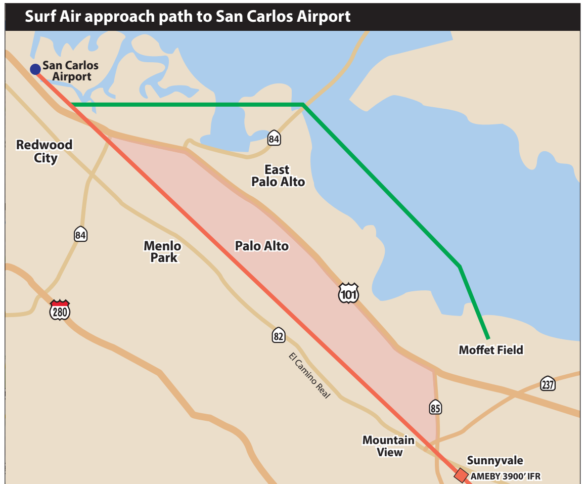
Surf Air says it will use a new approach route (green line) from near Moffett Field to the San Carlos Airport when conditions allow a visual flight rules (VFR) approach. The route that would continue to be used when visibility is poor is the straight line in orange. The shaded area is currently used by Surf Air pilots in VFR conditions.
