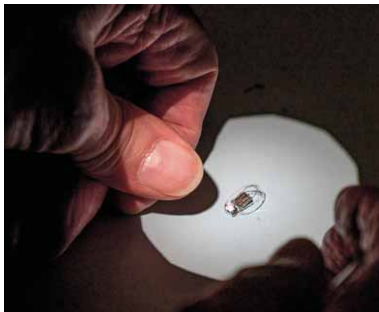
The tiny EarLens sits on the ear drum and helps amplify a wider spectrum of sound frequencies for its wearers than other hearing aids, Perkins says.
