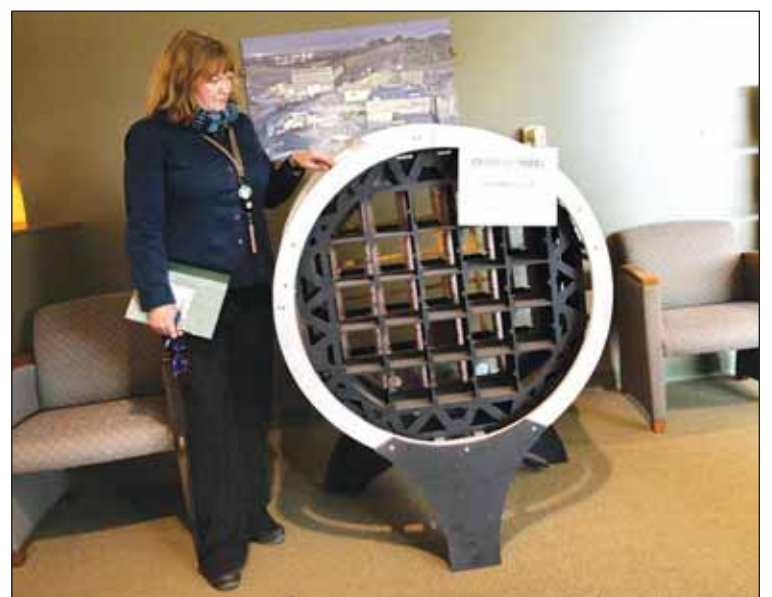
A model of the camera’s cryostat — a compartment designed to maintain extremely cold temperatures — includes a grid for mounting the camera’s sensors
